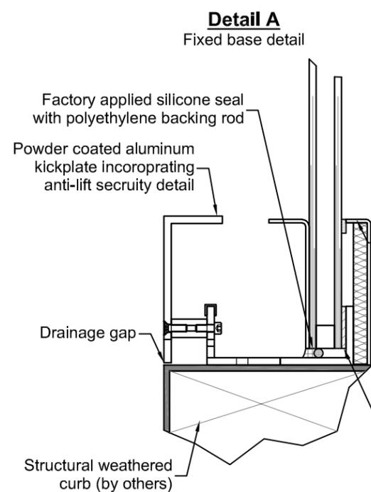
Minimum 1/4" drainage gap between curb and flooring required
